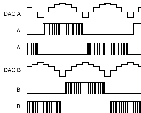
Figure 11: Stepper Motor Waveform - LM9832 Signals
